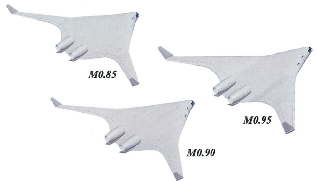
Fig. 38 Comparison of BWB-250 configuration with Mach number.
