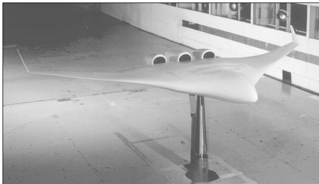
Fig. 15 Powered BWB model in the NASA LaRC 14 x 22 foot tunnel for low-speed test.
